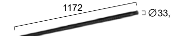
No 4317400 ● • 3000K LED 60W • 4095Lm No 4317410 ● • 4000K LED 60W • 4498Lm Beam Angle 24° • CRI >80 48V DC
